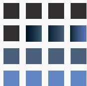
Sufficient temperature, time and steam penetration.
