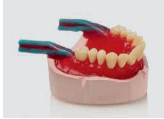
2. Addition of pouring channels and creation of orientation points on the model
