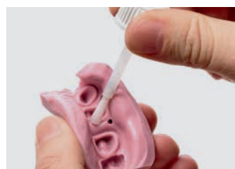
5. Creation of holes for silicone injection and application of the separator to the mask
