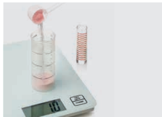
6. Weigh the resin, measure the monomer and mix, pouring the monomer in first and then the resin
