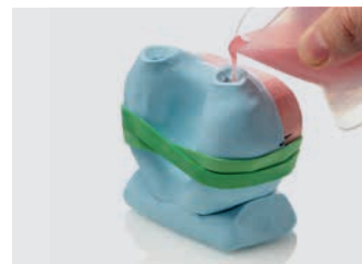
14. Pour the resin into one of the two pouring channels
