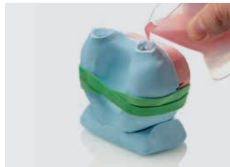
12. Pour the resin into one of the two pouring channels
