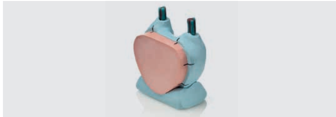
5. Base construction in Platinum 95 to keep the structure in a vertical position, marking of orientation points to check the correct repositioning of the silicone
